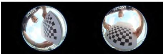
**Figure 1:** Checkerboard method for camera calibration
