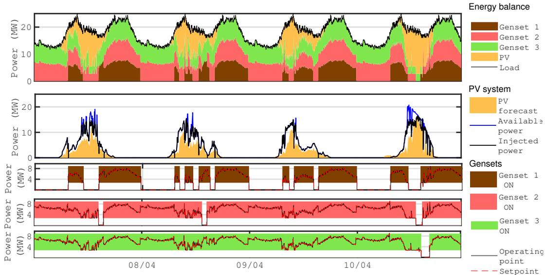
Fig. 5. Example of results for 4 days of simulation for strategy S2. From top to bottom: Energy balance in the system is represented, then available and injected PV energy, and below the operation the three gensets.
