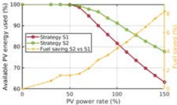
Fig. 6. Available PV energy injected (in percent) for different sizes of PV system (in percentage of the maximum load power). Fuel saving between strategy S2 and S1 is also represented (right axis). Results are obtained for 30 days of simulation.
