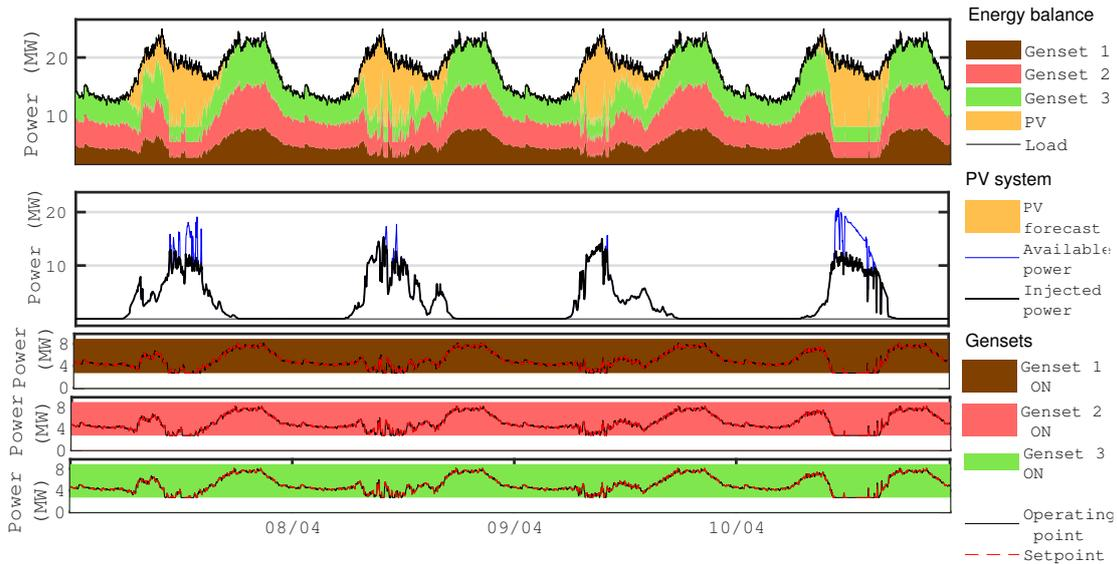
Fig. 4. Example of results for 4 days of simulation for strategy S1. From top to bottom: Energy balance in the system is represented, then available and injected PV energy, and below the operation the three gensets.
