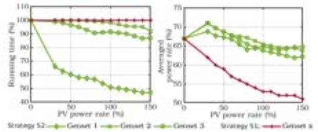
Fig. 7. Left: Operating time of the different gensets (in percentage of the total time). Right: Averaged operating rate of the genset nominal power. For both graphs, only one genset (genset x) is represented for strategy S1, as the three gensets have the same operating points
