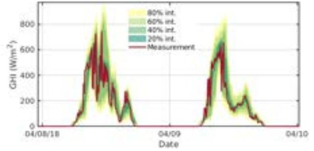
Fig. 2. Example of 2 days of GHI measurement at SteadySun test site, associated with their probabilistic short-term PV forecasts (horizon = 15 min)
